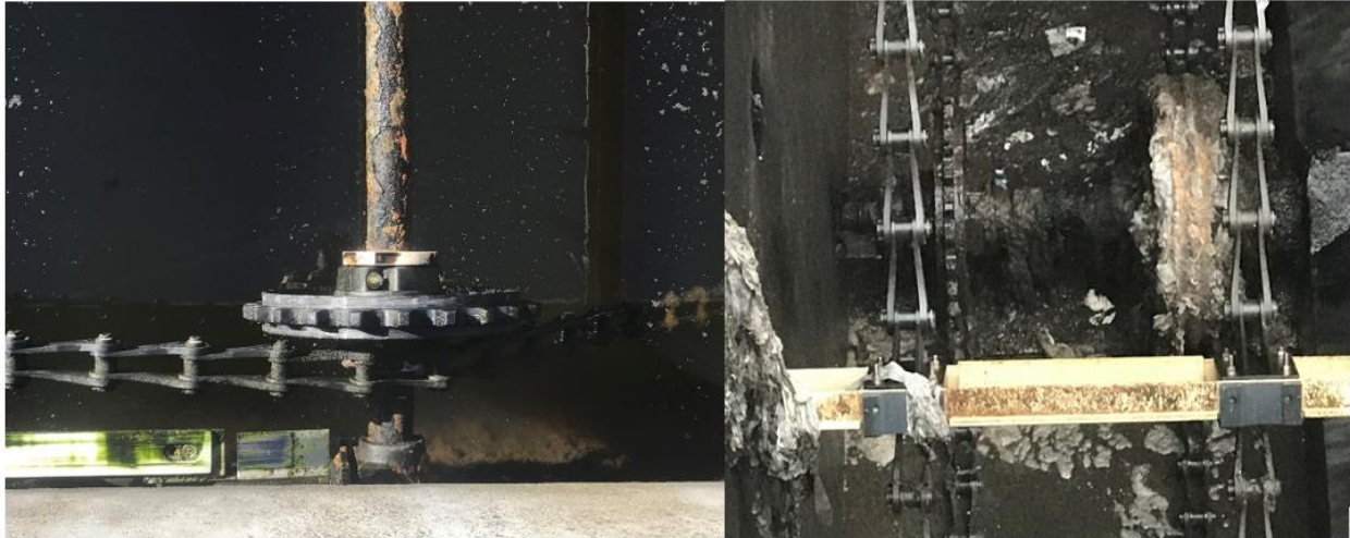
Figure 4 (Left) Chain jumped off the sprocket (Right) Sprocket covered with rags
