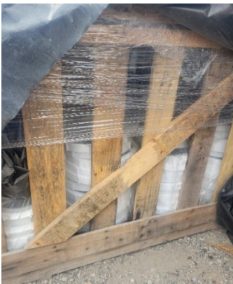
Disc diffusers for the aeration basins
