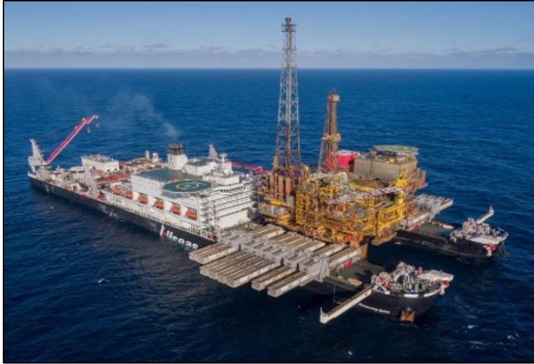
Figure 14. Pioneering Spirit transporting the Brent Delta topside (Shell 2019)
