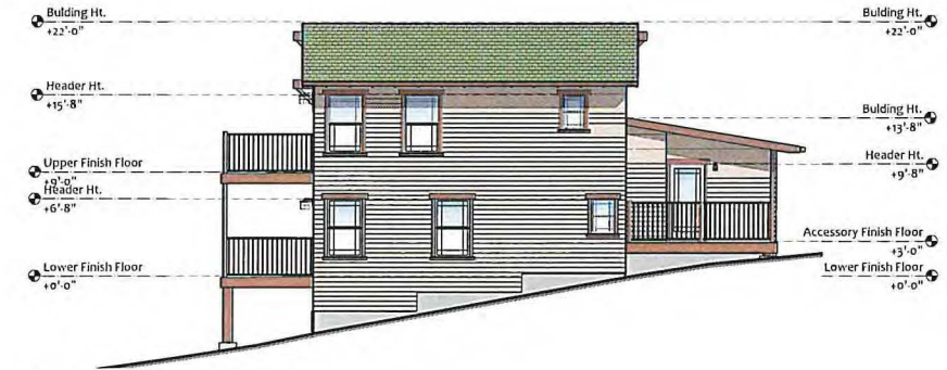
RIGHT ELEVATION (LEFT MIRRORED) Scale: 1/8" = 1'-0"
