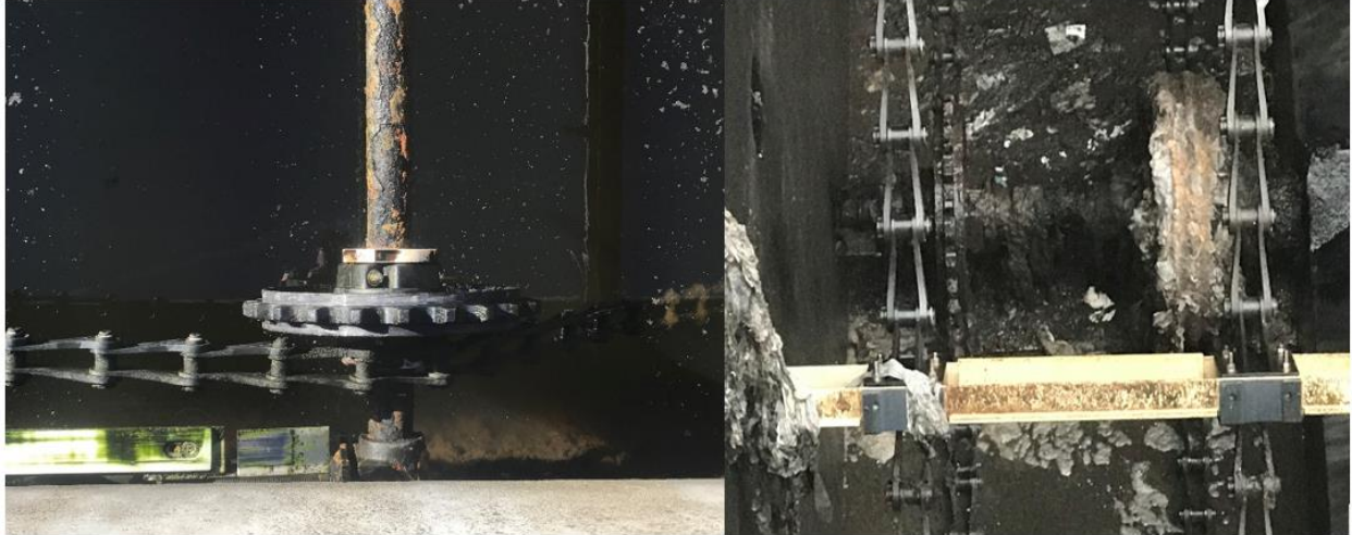
Figure 4 (Left) Chain jumped off the sprocket (Right) Sprocket covered with rags
