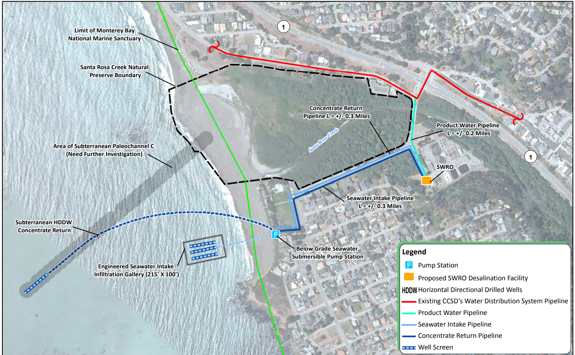
Figure 2.2.2-1 Water Supply Concept 2 Shamel Park Option 2 Facility Layout
