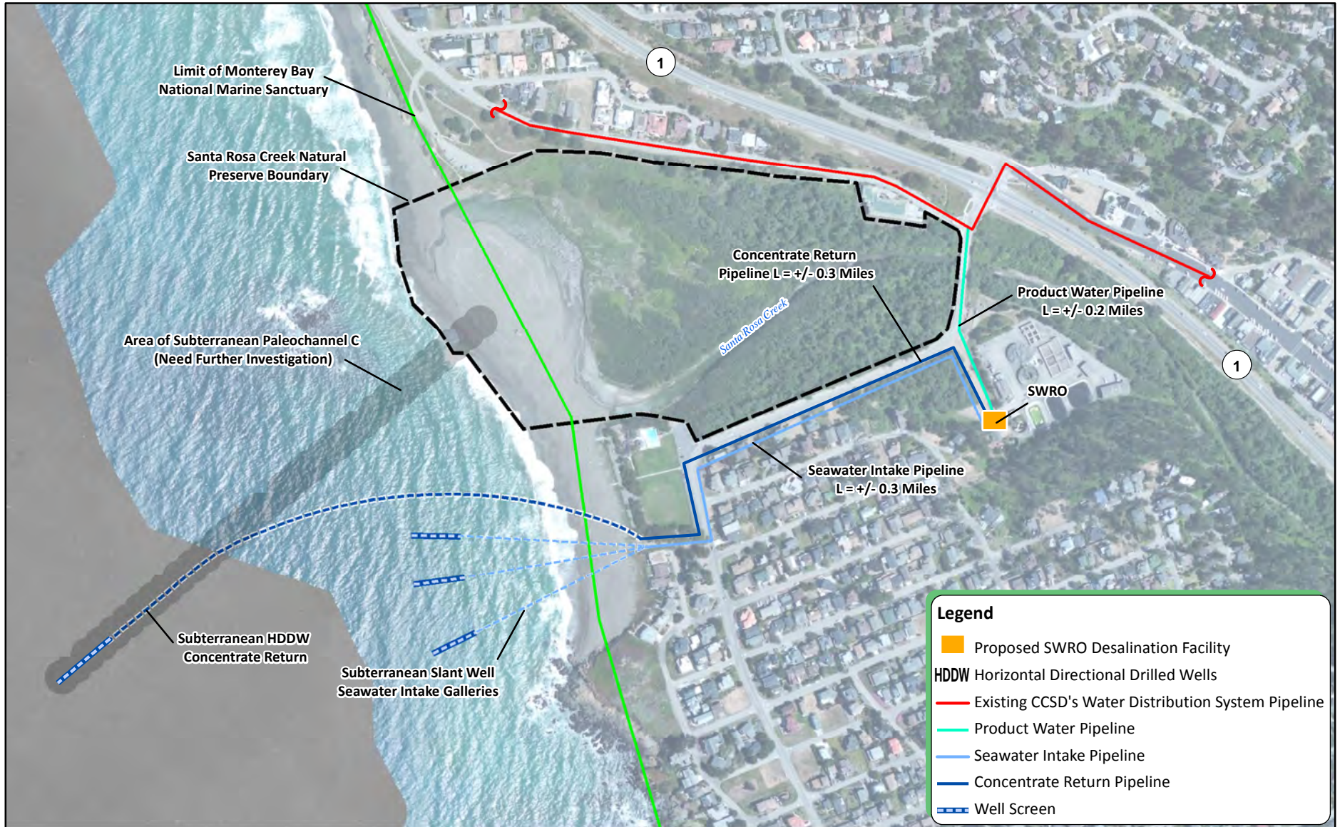
Figure 2.2.1-1 Water Supply Concept 1 Shamel Park Option 1 Facility Layout
