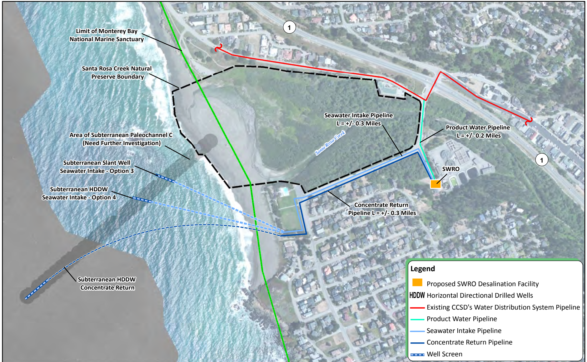
Figure 2.2.3-1 Water Supply Concepts 3 and 4 Shamel Park Options 3 and 4 Facility Layouts
