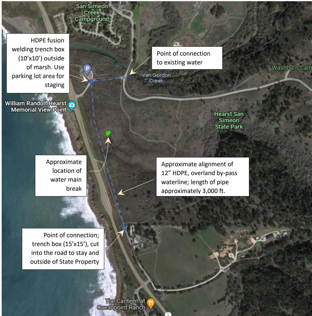
Figure 1- Site location of water main break and proposed repair
