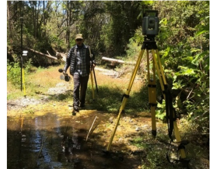
Topographic survey with total station in Santa Rosa Creek.
